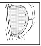
The instrument panel fuse block access door is located on the driver side edge of the instrument panel.
