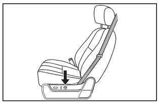
To increase lumbar support, press and hold the front of the control. To decrease, press and hold the rear of the control.
