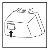
The light sensor is located on the inside of the vehicle in front of the inside rearview mirror.
