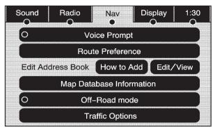
Press the CONFIG key to enter the configure menu options, then press the CONFIG key repeatedly until Nav is selected or touch the Nav screen button.
