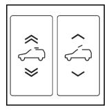
There are two switches in the overhead console that operate the sunroof.
