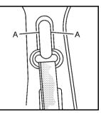
Squeeze the buttons (A) on the sides of the height adjuster and move the height adjuster to the desired position. The adjuster can be moved up just by pushing up on the shoulder belt guide.
