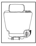
Lift the release lever, located on the bottom rear of the seatback on the outboard side of the seat, and the seatback will fold forward.
