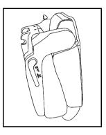
3. Lift the lever again to release the rear of the seat from the floor. The seat will tumble forward.
