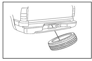
2. Tilt the tire toward the vehicle. Separate the tire/ wheel retainer (G) from the guide pin. Pull the pin through the center of the wheel. Tilt the retainer down and through the center wheel opening.
