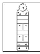
The power window switches are located on the driver door. In addition, each passenger door has a switch for its own window.
