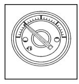
When the ignition is on, the fuel gauge shows about how much fuel the vehicle has left in the tank.
