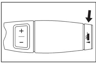
Pressing this button at the end of the shift lever turns on and off the tow/haul mode.
