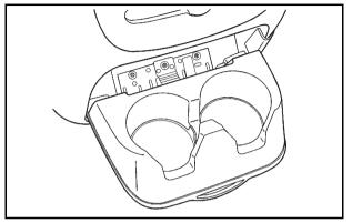
Pull down on the lid to access the cupholders in the rear floor console.
