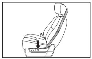
The controls used to operate the power lumbar feature are located on the outboard side of the seats.
