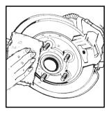
7. Remove any rust or dirt from the wheel bolts, mounting surfaces, and spare wheel.
