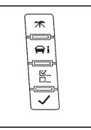
The DIC buttons are located on the instrument panel, next to the steering wheel.
