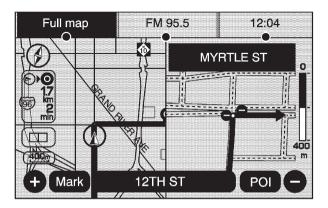
When approximately 1/4 mi (400 m) from the next maneuver, the screen displays the name and a detailed view of it.
