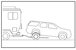
Use the following procedure to dinghy tow a two-wheel-drive vehicle from the rear:
