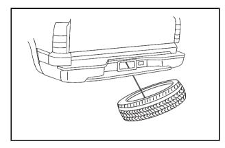
Tilt the tire toward the vehicle with some slack in the cable to access the tire/wheel retainer (G). Separate the retainer from the guide pin by sliding the retainer up the pin while pressing down on the latch.
