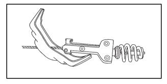
Once the retainer is separated from the pin, tilt the retainer and pull it through the center of the wheel along with the cable and latch.
