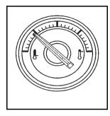
This gauge shows the engine coolant temperature.
