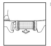
Unlatch the seat from the floor by pulling the carrying handle, located at the rear of the seat, rearward.
