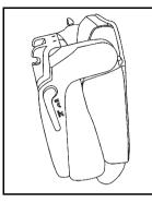
3. Lift the same lever again to release the rear of the seat from the floor. The seat will tumble forward. Folding and Tumbling the Seat(s) from the Third Row Seats
