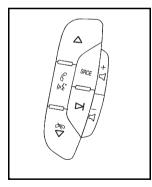
Audio steering wheel control functions could differ depending on the vehicle's options. Some audio controls can be adjusted at the steering wheel.  $\triangle$  /  $\nabla$ : Press to change favorite radio stations, select tracks on a CD/DVD, or to navigate tracks or folders on an iPod<sup>®</sup> or USB device.
