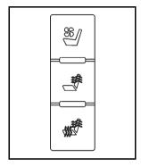
On vehicles with heated and cooled front seats, the controls are located on the climate control panel.
