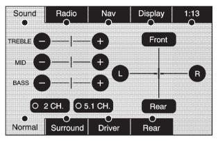
◆ (Sound): Press this key or press the CONFIG key to access the Sound menu to adjust the treble, midrange, bass, fade, balance, and Digital Signal Processing (DSP). The system automatically stores audio adjustment settings as changes are made for each audio source including AM, FM, XM (if equipped), CD, and AUX.
