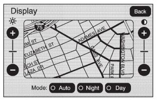
Touch this screen button to change the brightness, contrast, and mode of the display.
