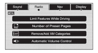
Press the CONFIG key to enter the configure menu screen, then press the CONFIG key repeatedly until Radio is selected or touch the Radio screen button to make changes for radio information displayed or to limit features while driving, number of preset pages, XM categories, and Bose<sup>®</sup> AudioPilot<sup>®</sup>.
