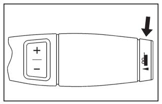
The vehicle has a tow/haul mode. The tow/haul mode adjusts the transmission shift pattern to reduce shift cycling, providing increased performance, vehicle control, and transmission cooling when towing or hauling heavy loads.
