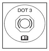
The brake master cylinder reservoir is filled with DOT 3 brake fluid. See *Engine Compartment Overview on page* 7-16 for the location of the reservoir.
