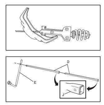
3. Assemble the two jack handle extensions (D) and wheel wrench (E) as shown.
