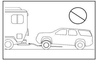
*Notice:* If a two-wheel-drive vehicle is towed with the rear wheels on the ground, the transmission could be damaged. The repairs would not be covered by the vehicle warranty. Never tow the vehicle with the rear wheels on the ground. Two-wheel-drive vehicles should not be towed with the rear wheels on the ground. Two-wheel-drive transmissions have no provisions for internal lubrication while being towed.
