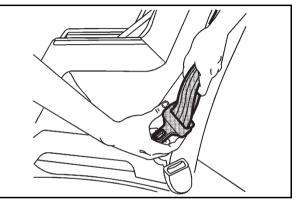
For third row seating positions, with cinching latch plates, tilt the latch plate to adjust the belt if needed.
