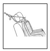
If the position you are using has an adjustable headrest or head restraint and you are using a dual tether, route the tether around the headrest or head restraint. 3. Push and pull the child restraint in different directions to be sure it is secure.
