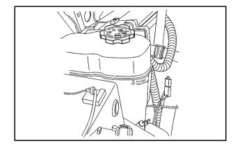
The coolant surge tank is located in the engine compartment on the passenger side of the vehicle. See *Engine Compartment Overview on page 7-16* for more information on location.
