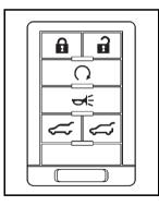
Press to unlock the driver door. Press a again within five seconds to unlock all remaining doors.
