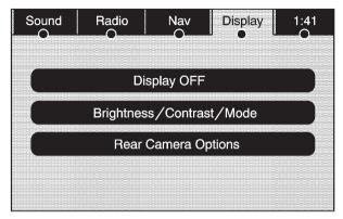
Press the CONFIG key to enter the configure menu options, then press the CONFIG key repeatedly until Display is selected or touch the Display screen button.
