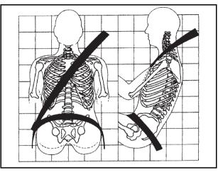
Sit up straight and always keep your feet on the floor in front of you. The lap part of the belt should be worn low and snug on the hips, just touching the thighs. In a
