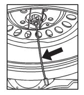
Check under the vehicle to see if the cable end is visible. If the cable is not visible proceed to Step 6.
