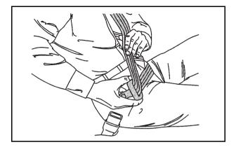
If the belt stops before it reaches the buckle, for lap-shoulder belts with cinching latch plates, tilt the latch plate and keep pulling the safety belt until it can be buckled.
