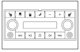
${\bf U}$  (Power): Press the  ${\bf U}$  button to turn RSA on and off.
