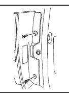
2. Remove the two screws from the taillamp assembly.
