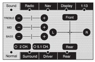
Press the CONFIG (Configure) hard key to adjust several of the system's features and preferences. The last selected CONFIG screen is the screen that displays: Sound, Radio, Nav (navigation), Display, or Time.
