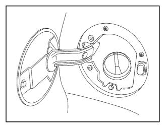
The tethered fuel cap is located behind a hinged fuel door on the driver side of the vehicle. If the vehicle has E85 fuel capability, the fuel cap will be yellow and state that E85 or gasoline can be used. See *Fuel E85 (85% Ethanol) on page 7-9.*
