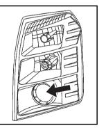
2. Locate the center of the projector lens of the low-beam headlamp.
