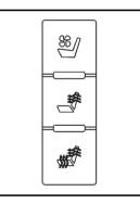
If the front seats have the heated and cooled seat feature, the buttons used to control this feature are located on the climate control panel.
