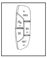
Cruise Control shown with Heated Steering Wheel Button (If Equipped) The cruise control buttons are located on left side of the steering wheel.
