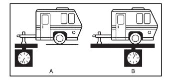
Trailer tongue weight (A) should be 10 percent to 15 percent and fifth wheel or gooseneck kingpin weight should be 15 to 25 percent of the loaded trailer weight up to the maximums for vehicle series and hitch type shown below:
