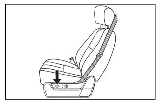
The power seat controls are located on the outboard side of the front seats.
