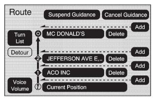
**Add Stopover:** Select this screen button from the Route screen. This feature allows up to three stopovers to be added to the current route between the start point and final destination. Once a stopover has been added, the points can be edited or deleted.
