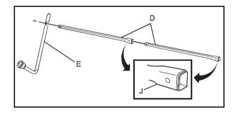
4. Assemble the two jack handle extensions (D) and wheel wrench (E) as shown.
