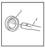
Insert the open end of the extension (J) through the hole in the rear bumper (I) (hoist shaft access hole). Be sure the hoist end (J) of the extension (D) connects to the hoist shaft (B). The ribbed square end of the extension is used to lower the spare tire.
