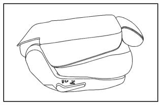
The seatback will fold forward automatically. Leaving the seatback in this position creates a flat load floor.
