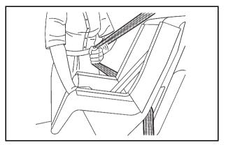
4. For passenger seating positions with a lap-shoulder belt and a free-falling latch plate, pull the rest of the shoulder belt all the way out of the retractor to set the lock. When installing a child restraint using a lap-shoulder belt and a cinching latch plate, skip Step 4 and proceed to Step 5.
