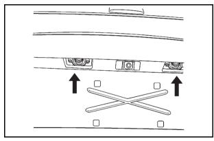
1. Remove the two screws holding each of the license plate lamps to the molding that is part of the liftgate.
