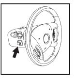
The power tilt wheel control is located on the left side of the steering column.
