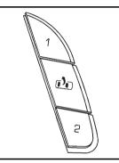
The controls for this feature are located on the driver's door, and are used to program and recall memory settings for the driver's seat, outside mirrors, steering wheel position, and the adjustable throttle and brake pedal feature, if your vehicle has it. To save your positions in memory, do the following:
