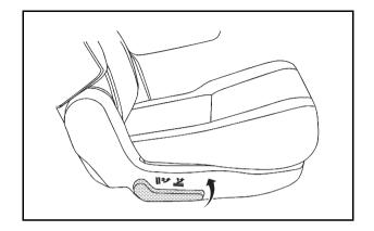
2. Lift the lever, located on the outboard side of the seat, to release the seatback.
