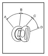
The ignition switch has four different positions.
