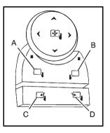
Controls for the outside power foldaway mirrors are located on the driver door armrest.
