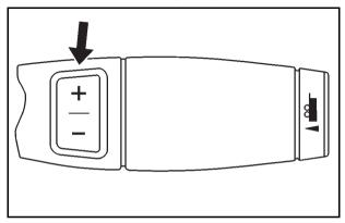
The vehicle has Driver Shift Control (DSC). DSC controls the vehicle's transmission and vehicle speed while driving down hill or towing a trailer by allowing you to select a desired range of gears.
